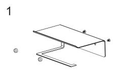
Plug the screw holes with the threaded screw and thread the decorative cap onto the plugged screw
