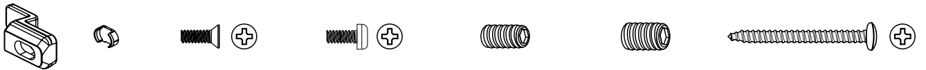
[15] x1 [16] x1 [17] x2 (M4x10) [18] x1 (M4x8) [19] x1 (M4x5) [20] x2 (M6x5) [21] x8 (ST4x35)
