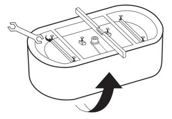
Turn the bath over and temporarily place in what will be final position in the bathroom.Check along the top of the bath using a spirit level and adjust the feel if necessary and lock into place.
